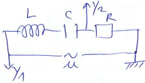
$$\begin{aligned} 2/ \quad a - \quad U_m &= Z I_m \\ U_{Rm} &= R I_m \end{aligned} \quad \left. \begin{array}{l} \\ \end{array} \right\} Z > R \Rightarrow U_m > U_{Rm}$$
